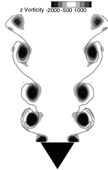
Fig. 2 Instantaneous image of the flame sheet (solid line) and vorticity isocontours [22].
